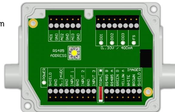
The industrial process interface offers the following inputs and outputs:
